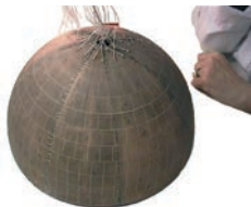
300 mm diameter half sphere transducer. Matrix array with more than 1000 elts.
