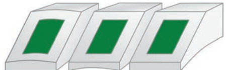
Customized contact face geometry to fit inspected parts or wedge focusing
