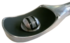
High power focused transducer for prostate cancer treatment
