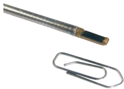
Miniature endoscopic probe combining imaging and high power capability on a single transducer
