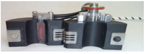
The Eddy Current Array (ECA) method is perfectly suited for Friction Stir Weld inspection. The welding bead is stable enough to avoid problems related to strong liftoff variations. While soldering, fissures can occur. The ECA method can detect tiny 250  $\mu$ m deep and 1 mm long fissures.
